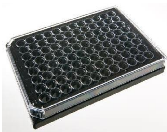
Fig. 5. Showing 96 well black bottom plates.
